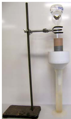
Figure 2.3 Measurement of saturated hydraulic conductivity using a constant head apparatus
