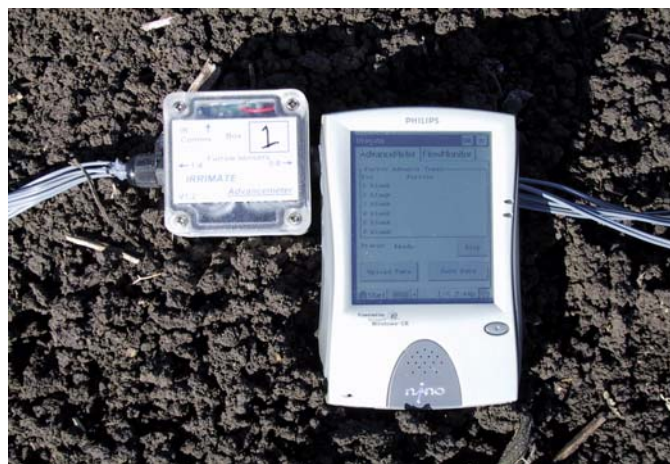
Figure 18: Irrimate furrow advance monitoring hardware and download device
