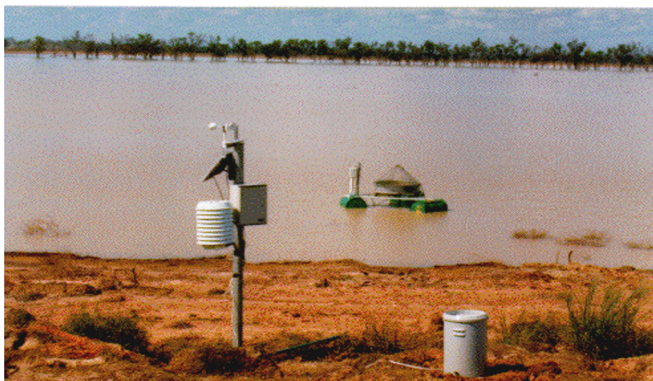
Figure 4: Weather Station and logged rainfall and evaporation pan sensors monitoring conditions at storage
