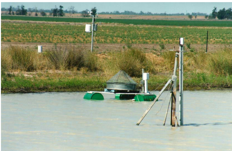
Figure 3: Storage monitoring equipment including weather station and logger (far left on bank); floating evaporation pan (middle) and shaft encoder water level instrument (near right)
