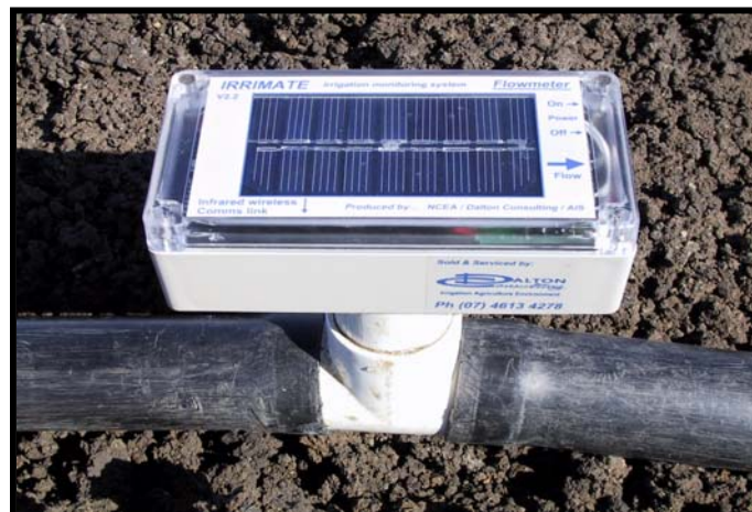
Figure 17: Irrimate siphon flow-monitoring hardware
