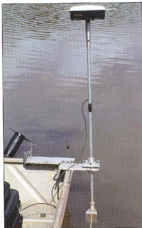
GPS antenna mounted above the electronic depth sounder.
