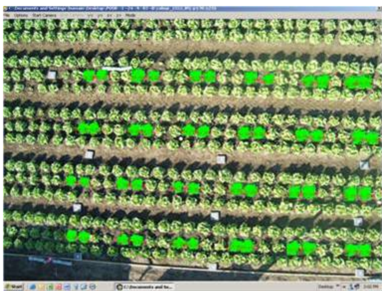
Figure 3. Example of an image acquired using the camera mounted on a 10 m mast and offset boom showing the green pixel mask of the physically measured plants.
