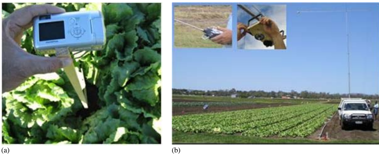
Figure 1. Image acquisition of the lettuce plants using digital cameras mounted at (a) 1.15 m and (b) 10 m above the ground surface
