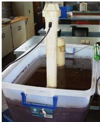
Figure 1: Capacitance sensors installed in a soil bin with water quality treatment being applied.
