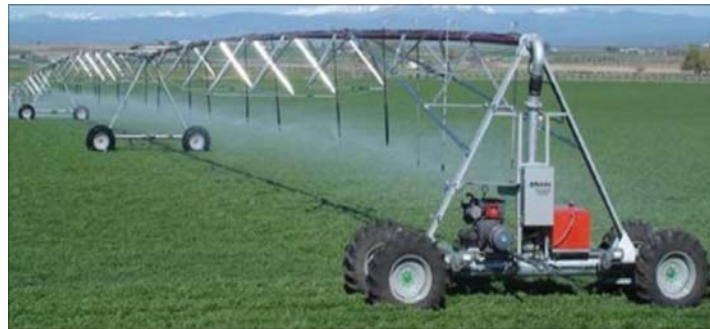
Fig. 1. Spans (gantries) of a lateral move irrigation machine (from CI 2010).
