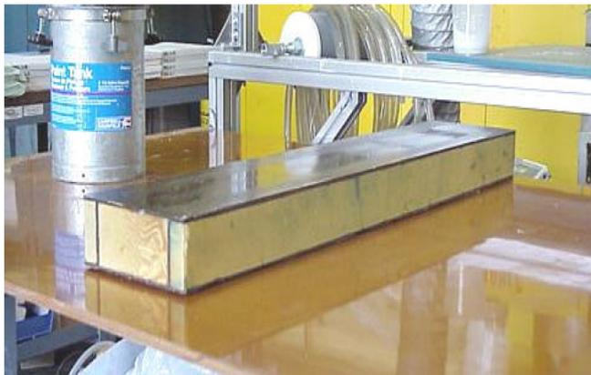
Figure 3. Natural fibre composite unit beam [42].
