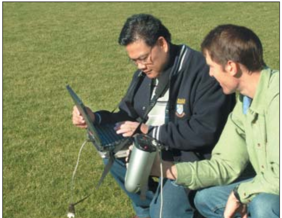
CLOSE EXAMINATION: Coordinator of the Geospatial Information and Remote Sensing Group and Senior Lecturer from the Faculty of Engineering and Surveying, Dr Armando Apan and Research Scientist with the Department of Primary Industries and Fisheries (DPIF), Dr Rob Kelly test the ASD hyperspectral sensor to determine the best spectral bands for remote sensing of grain protein content.
