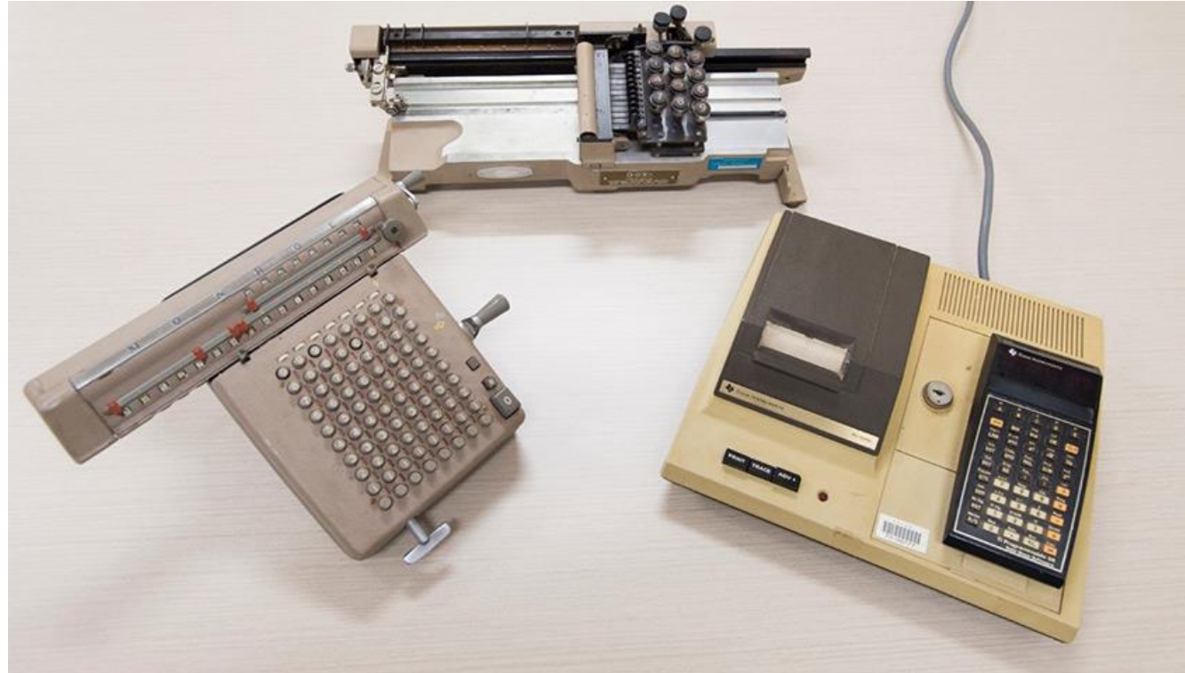
Mechanical calculator Monroe LN-160X (circa 1950), ICT Hand-operated card punch (circa 1960), TI59 Calculator with PC-100A print/security cradle (1977).
